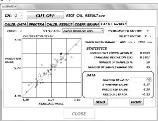
\* When a marker on the graph is clicked, data such as data number, standard value, predicted value, and residual error will be displayed in the data field on the right.
