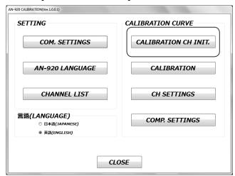
2 Initialize the channels for making the calibration curve. Select a channel, and click the [CALIBRATION CH INT.] button.
