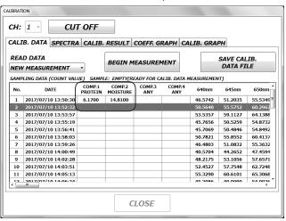
Enter the standard values of all the samples to be used in the regression calculation.
