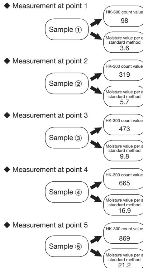
(3) Record the measurement results in count mode (calibration curve number 10) as in Table 1. (Please copy and use the "Calibration Curve Preparation Table" on p. 37.)
