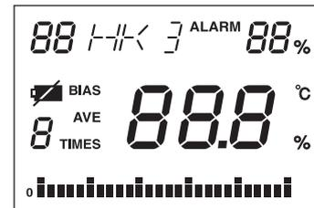
(2) Select a calibration curve from the included "calibration curve list." Press the **SELECT WX** key, and the calibration curve number will start blinking. Enter a 2-digit calibration curve number.
